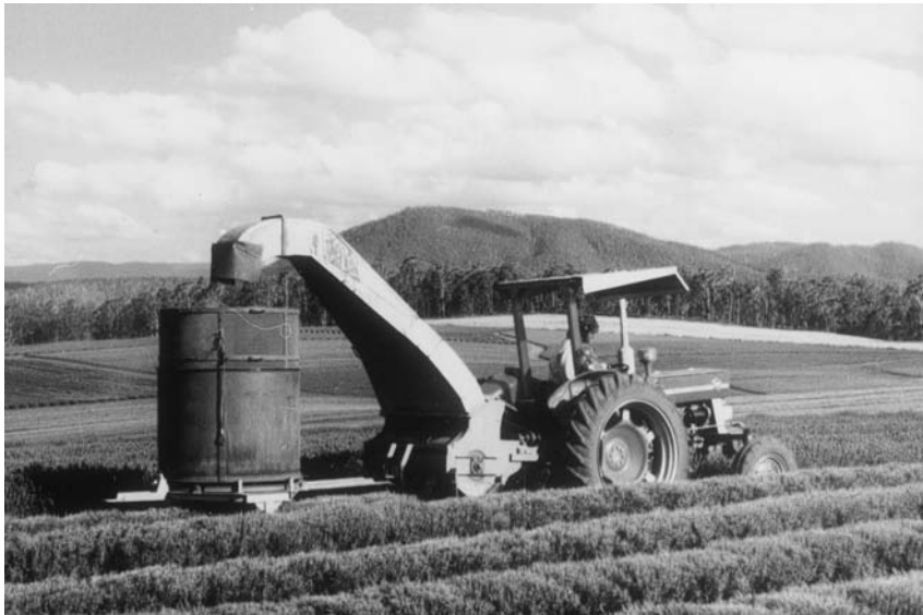
Figure 10.2 Harvesting at about two tons lavender flowers per hour.
